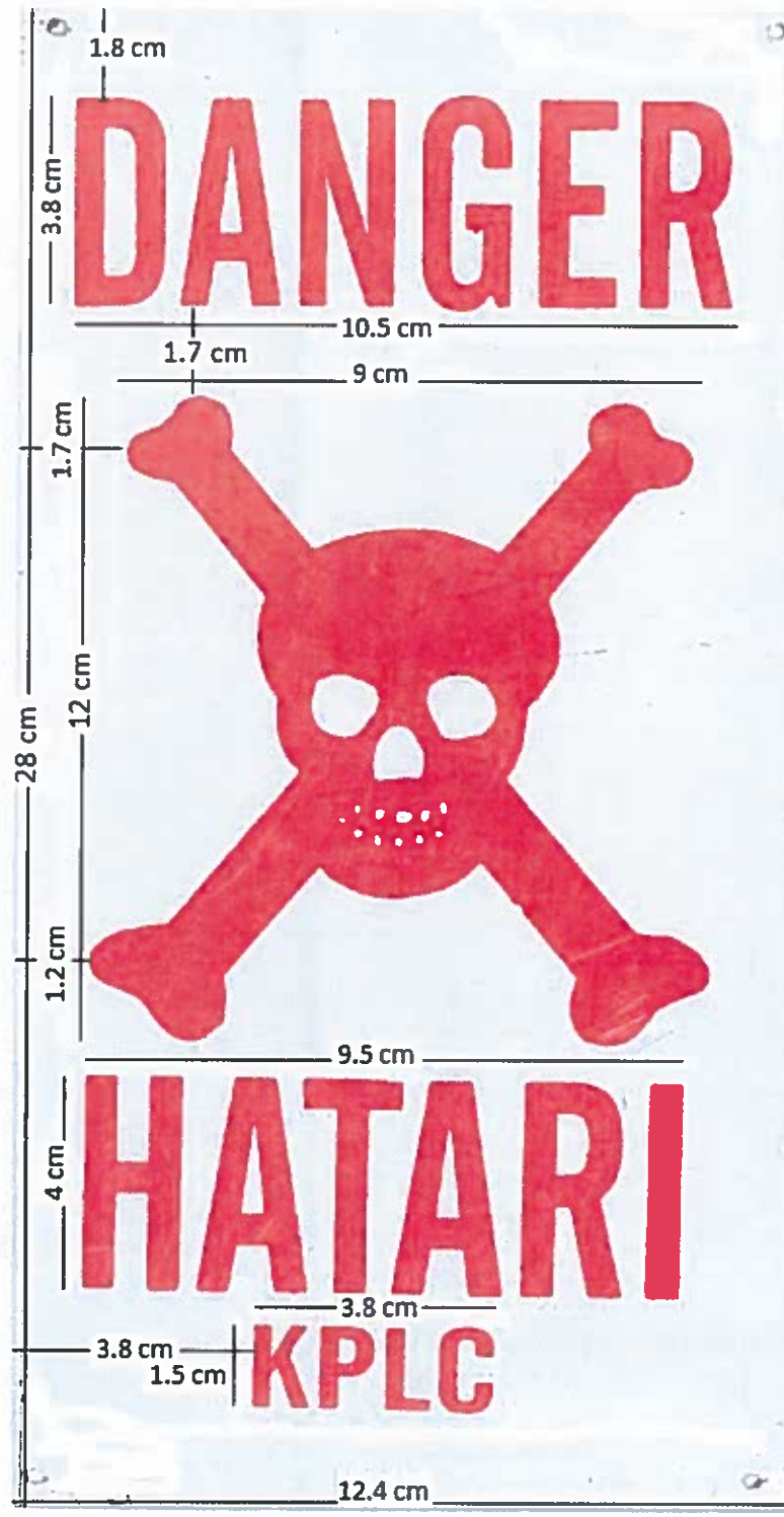
Fig. 3: Danger/Hatari plate for power lines
