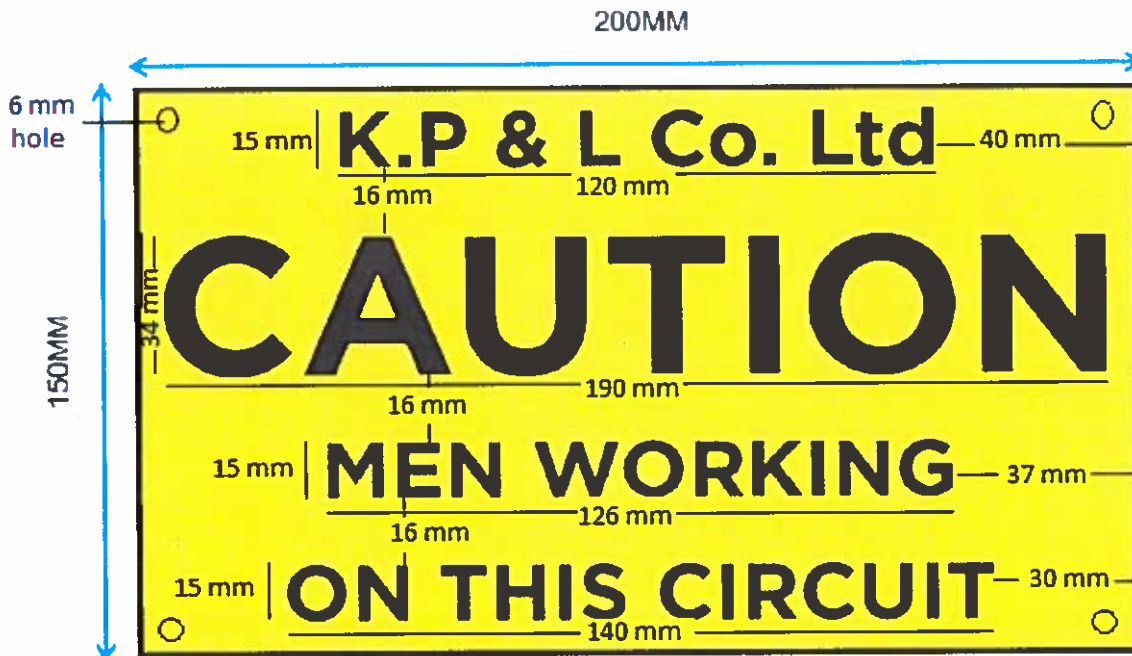
Fig. 7: Caution Notice Plate
